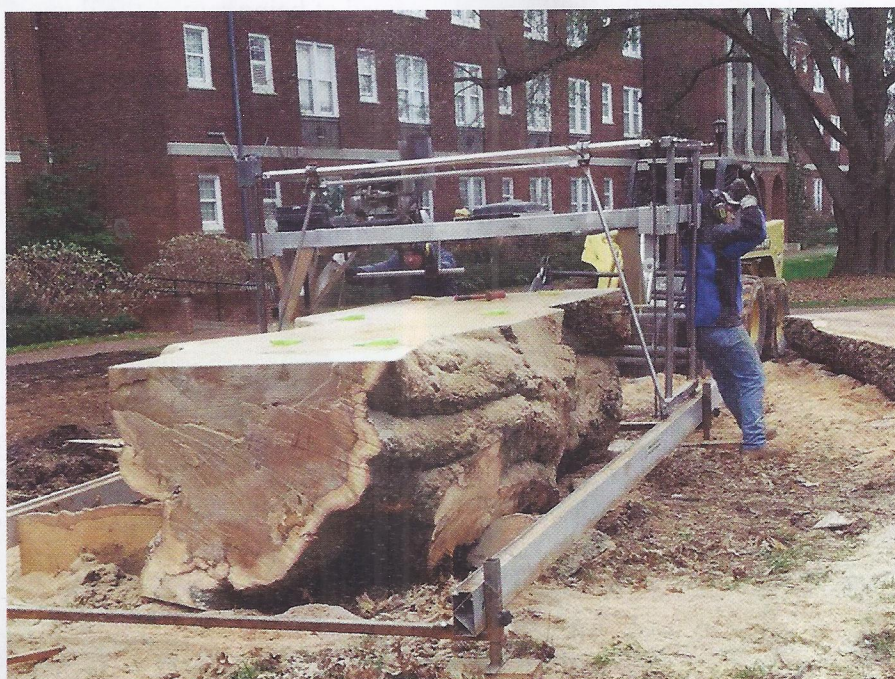
Slabbing blade at work on a log at Meredith College.
