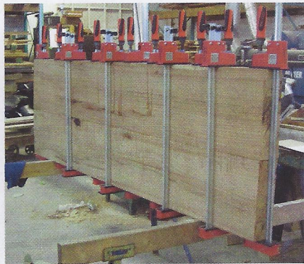
Left to right: glued bench tops made from slab stock; Grizzly resaw producing veneer from cants; and crane placing a 43-ft.-long log for sawing.
