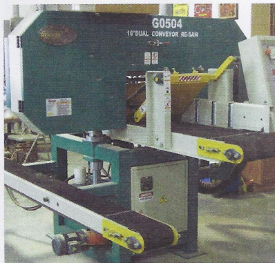
Left to right: glued bench tops made from slab stock; Grizzly resaw producing veneer from cants; and crane placing a 43-ft.-long log for sawing.
